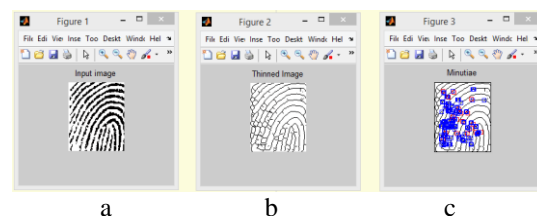
Fig. -3: a) Input fingerprint image b) Fingerprint image after thinning c) Minutiae extracted from the fingerprint image
