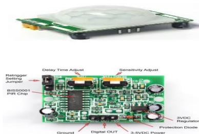
Fig. 3.4 Passive Infrared Sensor (PIR Sensor)
