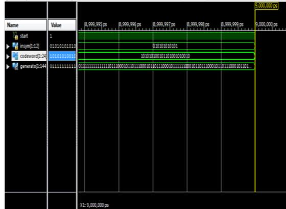
Figure 8 Encoding using Golay (24, 12)
