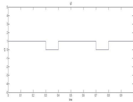
Fig. 15. Switching pattern for Q3
