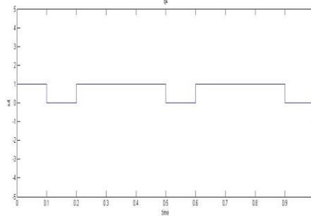
Fig. 16. Switching pattern for Q4
