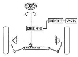
Figure 1: Rack and pinion steering gear
