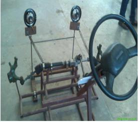
Figure 2: Steering System with movable headlights
