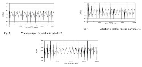
Fig. 5. Vibration signal for misfire in cylinder 4.
