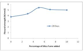
Fig. 4: Flexural strength of GPC Vs % of Silica fumes added
