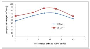
Fig. 3: Compressive strength of GPC Vs % of Silica fume at 7 and 28days
