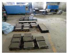
Fig. 1: Cubes and prisms casting
