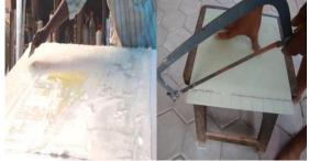
Fig. 1: Fiber Glass Epoxy Being Applied Evenly Layer By Layer(130rientation)
