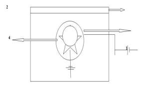
Figure 6: Layout of the system 1. Battery, 2. Polystyrene Box Or Thermocol Box, 3. Hole for Exhaust Fan, 4. Exhaust Fan, 5. Earth Connection.
