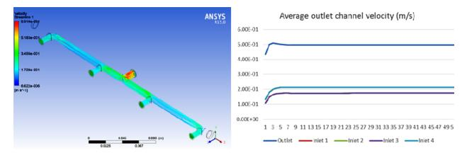
Fig. 3(a): Velocity Streamlines and outlet contours of the outlet channel, (b) Comparison of average outlet channel velocities
