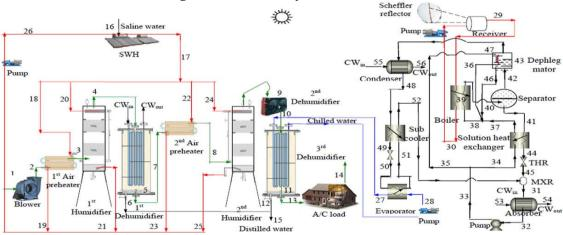
Fig. 1: Two-Stage Humidification Dehumidification Plant schematic (Chiranjeevi and Srinivas, 2014)
