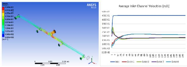
Fig. 2 (a): Velocity Streamlines and outlet contours of the inlet channel, (b) Comparison of average inlet channel velocities.
