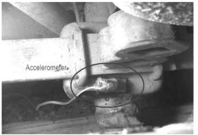
Figure 1. MEMS Accelerometer fixed on the axel
