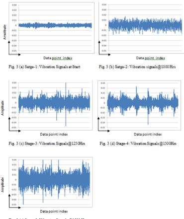
Fig. 3 (e) Stage-5: Vibration Signals @1800 Hrs.
