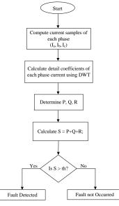
Fig. 2. Flowchart for fault detection algorithm
