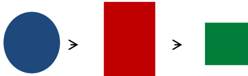
Fig.1: Transformation of a x^2+y^2 \leq a^2 in x-y plane to the rectangle 0 \leq r \leq a, 0 \leq \theta \leq 2\pi in r- \theta plane and then to a square 0 \leq \xi \leq 1, 0 \leq \eta \leq 1 in \xi - \eta plane
