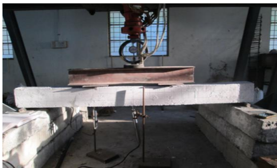
Fig -6 Testing of RC Beam (80% Sea sand)
