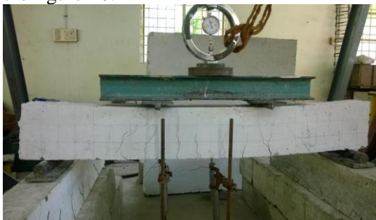
Fig-10 Failure pattern of the conventional beam
