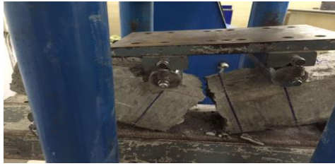
Fig. 2. Flexural failure of M2 proportion
