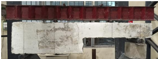
Fig. 5(d). Loading pattern for Type 2 SCC beam
