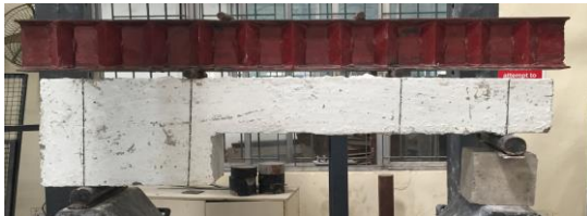
Fig.5(b). Loading pattern for Type 1 SCC beam
