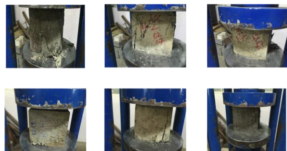
Fig. 1. Compressive failure for Six proportions Prisms of 500x100x100mm are casted for six different proportions and cured for 28 days, then tested to obtain optimum percentage for SCC
