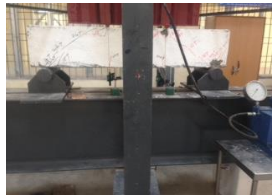
Fig.3(b): Cracks formed while testing RCC beam
