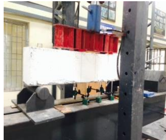
Fig. 3(a): RCC beam under cyclic loading arrangement
