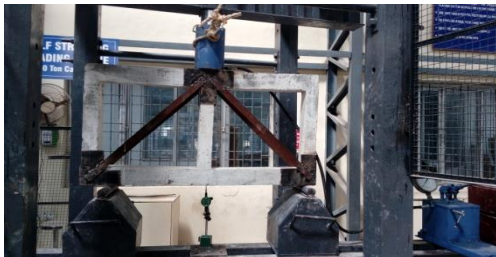
Fig 2.2: Strut welded along tested frame beam column joint
