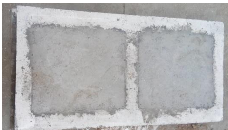
Fig 2.3 tested frame with concrete infill
