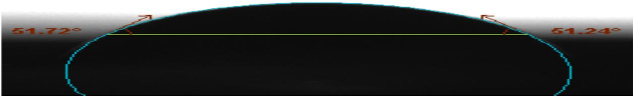
Fig. 7: Contact angle of pure PLA and PLA/Thymol/Graphene composites
