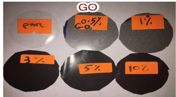
**Fig 2:** Samples of test of pure PLA and PLA/thymol/Graphene composites
