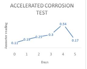
Graph 1: Result for accelerated corrosion test
