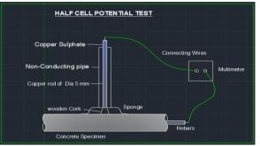
Fig. 4. Half-cell potential test
