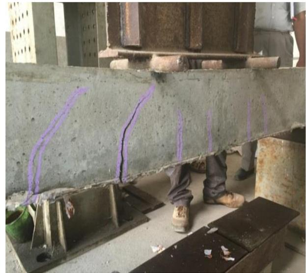
Fig. 2: Experimental test setup for SCC composite beam
