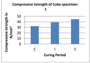
Fig. 1: Compressive strength of Cube specimen-1
