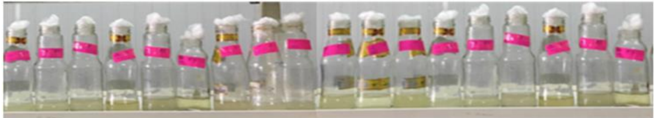
Figure 3. A. Fumigatus growing in MSM added diesel (10, 20 and 30 g/L) and control during (14, 21 and 28 days)
