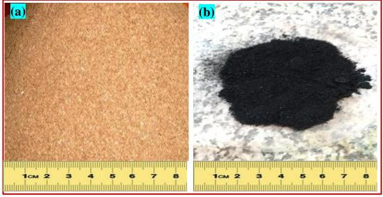
Figure 1: The sawdust waste (a) before burn (b) after burn.
