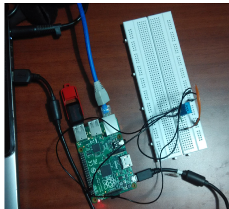
Fig. 7 Interfacing DHT 11 Sensor with Raspberry-Pi
