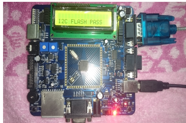
Figure.2 I2C Test result displayed in LCD
