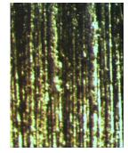
Fig. 1: The surface of the steel samples after mechanical processing (× 100).
