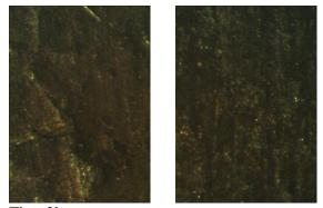
Fig. 2b: The surface of steel after incubation in the medium: oil – water - SRB (×100).
