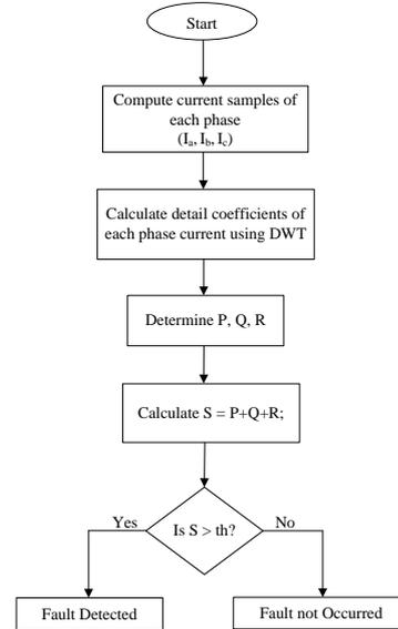
Fig. 2. Flowchart for fault detection algorithm
