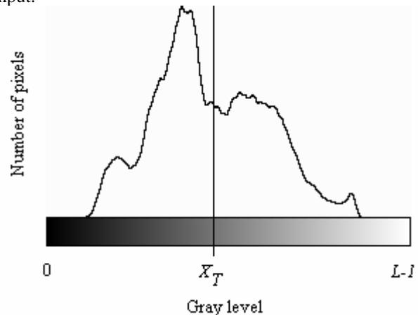
Fig. 3: Brightness preserving Bi Histogram Equalization [2]
