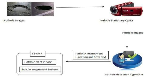
Figure 2: Pothole Detection System
