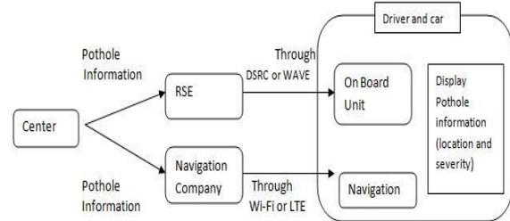
Figure 3: Pothole Alert System
