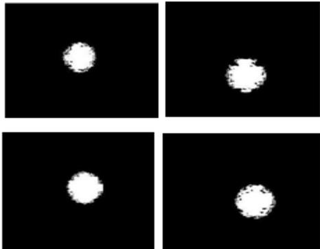
Fig. 9 The pupil region segmentation using Multiple Threshold Method with threshold value of  $\pm 2$
