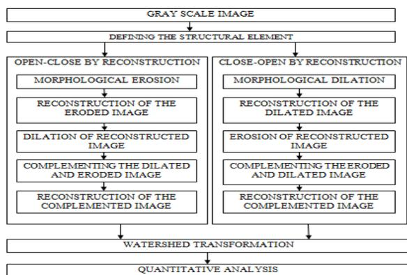
Fig. 3 Workflow of the Open-close and Close-Open Reconstruction process
