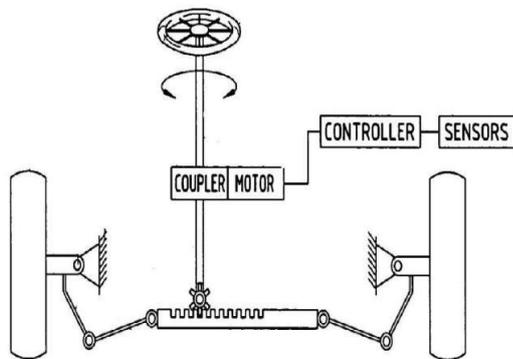
Figure 1: Rack and pinion steering gear
