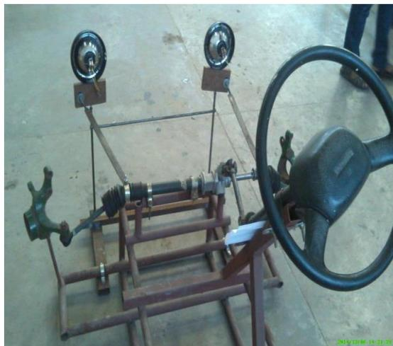
Figure 2: Steering System with movable headlights
