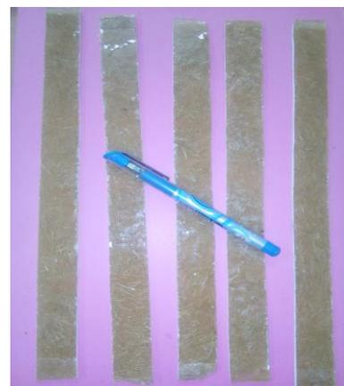
**Figure 1:** Digital images of composite specimens for the tensile test
