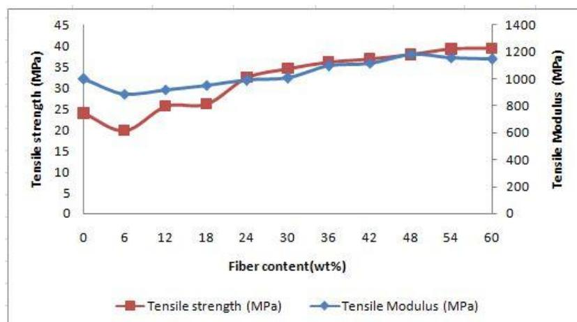
**Figure 2** Effect of fiber content on the tensile properties
