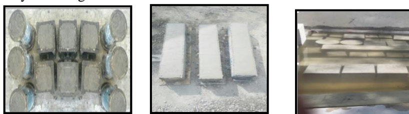
Figure 3: Casting Cubes, Cylinders, Beams & Curing
