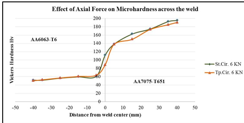
Figure 3: Influence of axial force on Micro-hardness
