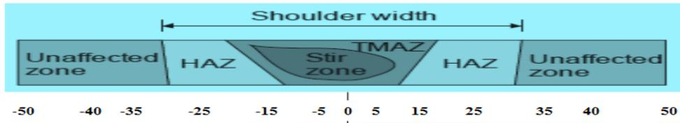
Figure 1: Micro-hardness measurement locations
