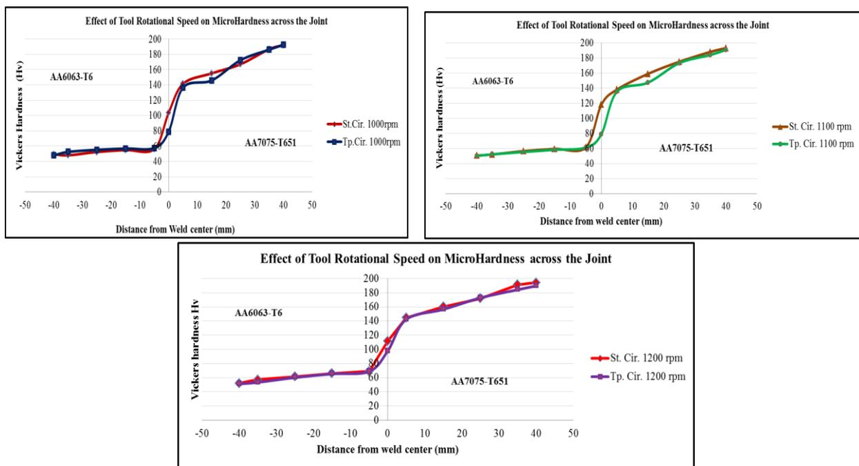
Figure 2: Influence of Tool revolving speed on Micro-hardness
