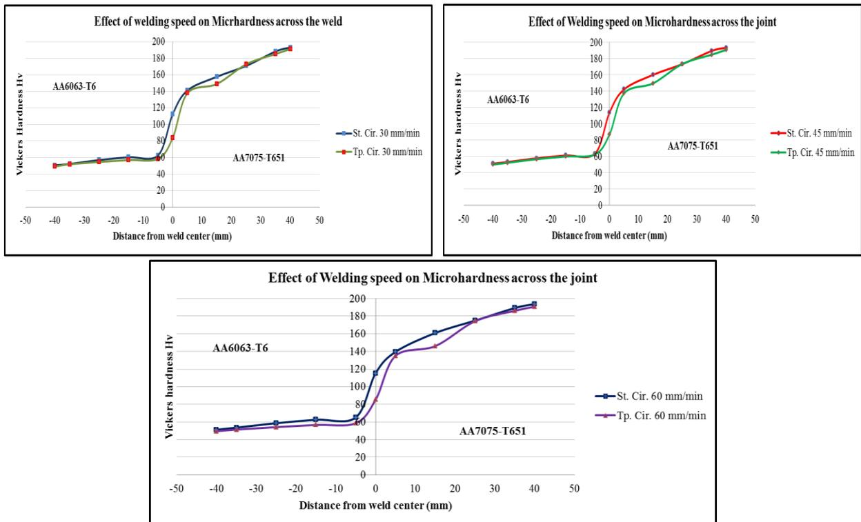
Figure 4: Influence of Welding Speed on Micro-hardness
