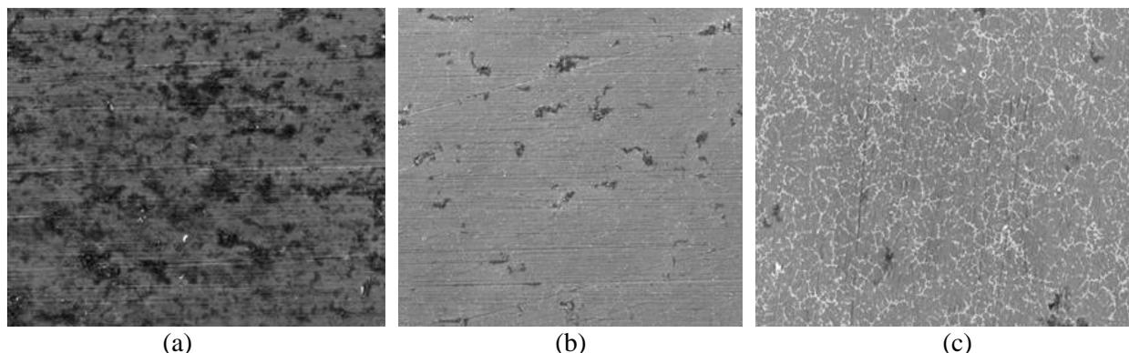
**Fig. 2:** SEM micrographs of corroded surface of (a) Pure Mg,(b) AZ31 and (c) AZ91 before in 3.5% NaCl concentration
