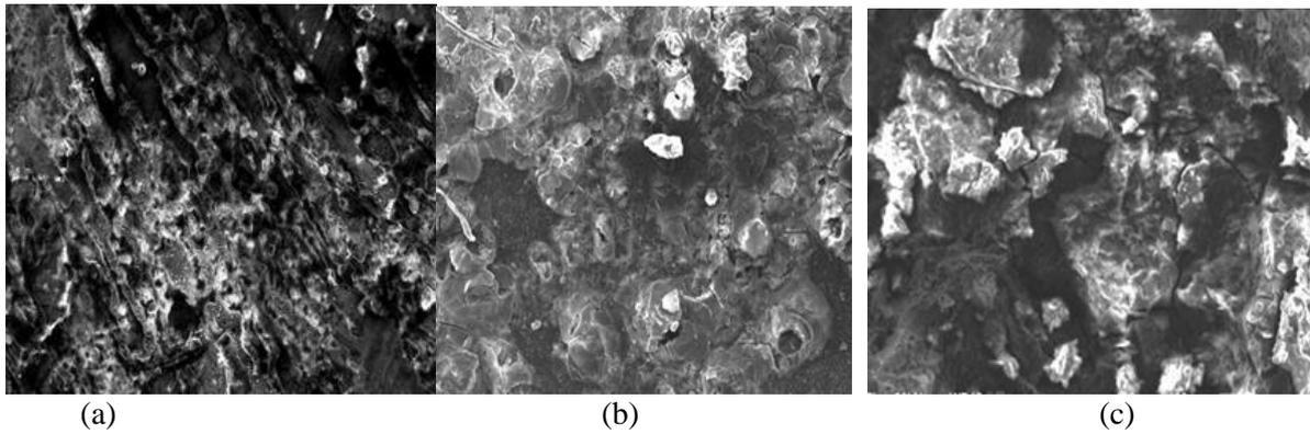
**Fig. 3:** SEM micrographs of corroded surface of (a) Pure Mg, (b) AZ31 and (c) AZ91 after exposure in 3.5% NaCl concentration in immersion test
