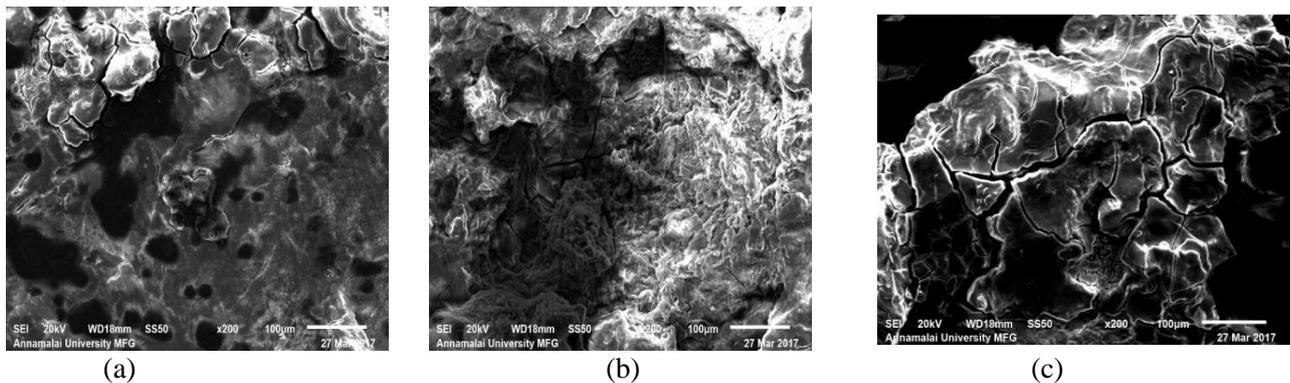
**Fig. 4:** SEM micrographs of corroded surface of (a) Pure Mg, (b) AZ31 and (c) AZ91 after exposure in 3.5% NaCl concentration under erosion corrosion process
