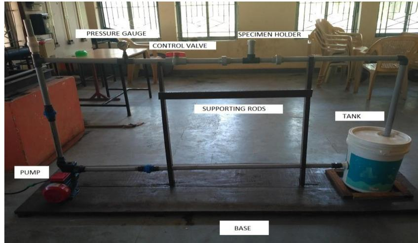
**Fig.1.** Experimental test rig for erosion corrosion
