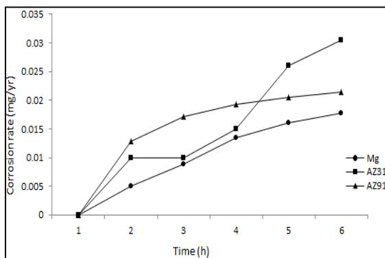
**Fig. 5** Corrosion rate vs time
