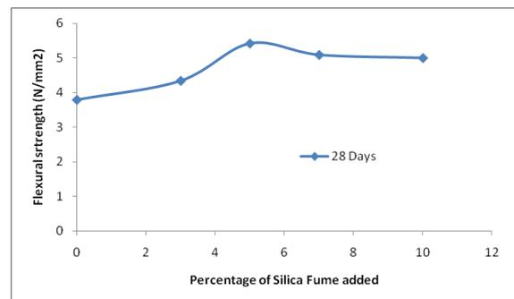
**Fig. 4: Flexural strength of GPC Vs % of Silica fumes added**
