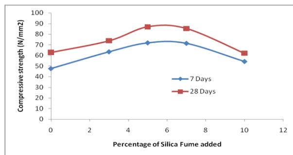
**Fig. 3: Compressive strength of GPC Vs % of Silica fume at 7 and 28 days**
