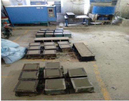
**Fig. 1: Cubes and prisms casting**
