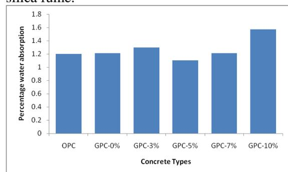
**Fig. 5: Water absorption of GPC Vs % of Silica fumes added**
