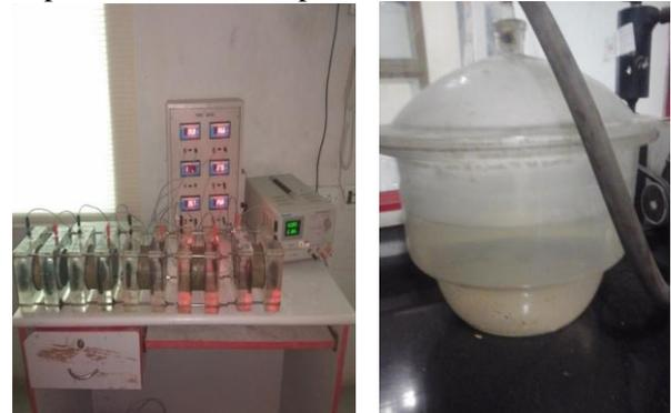
**Fig. 2: RCPT Experimental setup**
