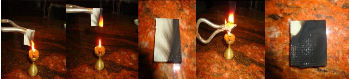
Fig. 3: Fiber Glass Epoxy laminate flammability rating
