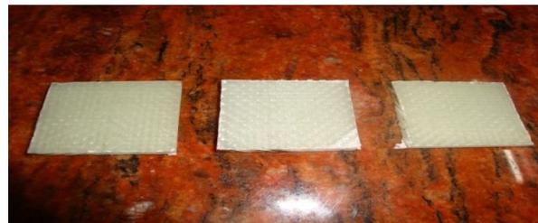
Fig. 2: Laminate Being Cut In To Pies For Chemical And Famablaty Testing
