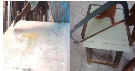
Fig. 1: Fiber Glass Epoxy Being Applied Evenly Layer By Layer(13Orientation)
