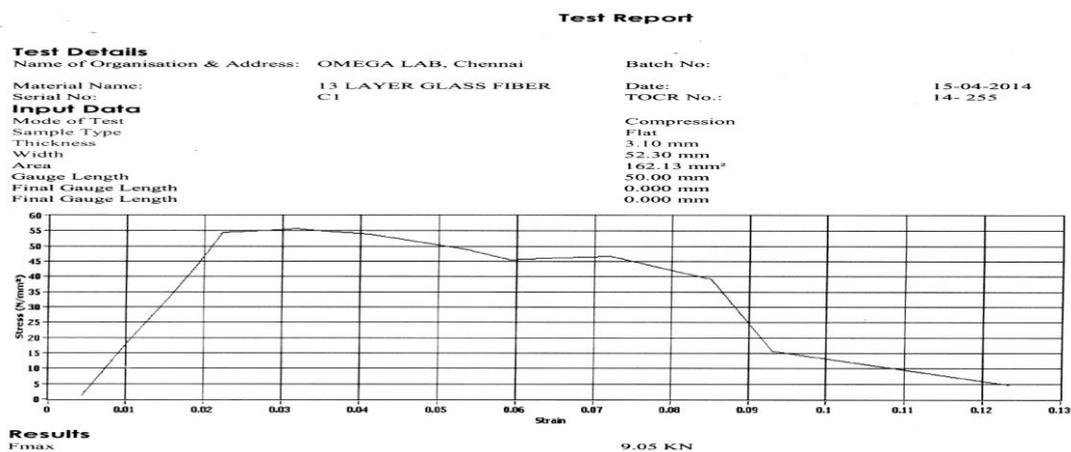
Fig. 4: Stress Vs Strain for 13- layer orientation glass fiber laminate
