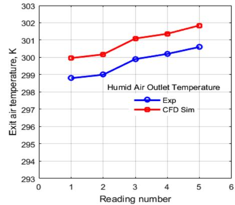
Fig. 4a: Comparison of coolant water outlet temperature, (b) Comparison of humid air outlet temperature.
