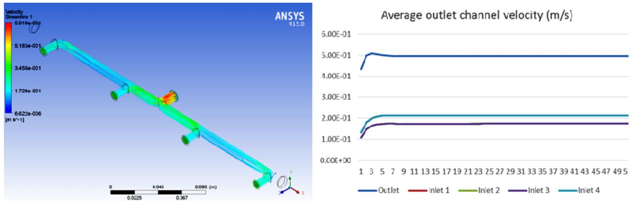
Fig. 3(a): Velocity Streamlines and outlet contours of the outlet channel, (b) Comparison of average outlet channel velocities
