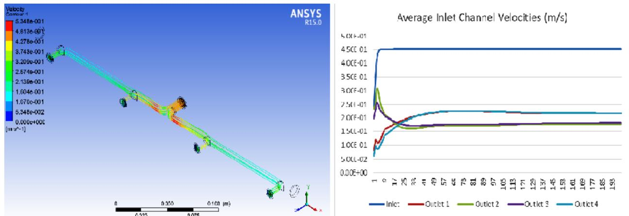
Fig. 2 (a): Velocity Streamlines and outlet contours of the inlet channel, (b) Comparison of average inlet channel velocities.
