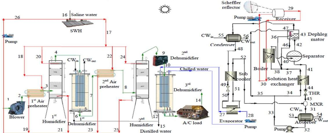
Fig. 1: Two-Stage Humidification Dehumidification Plant schematic (Chiranjeevi and Srinivas, 2014)
