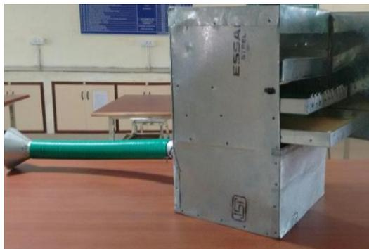
**Figure-2:** Fume Extraction and Filtration Equipment
