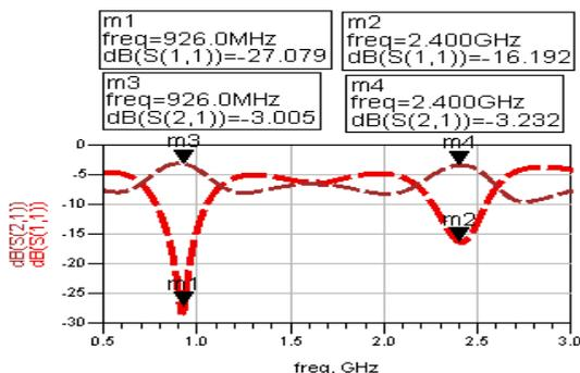
Figure-4: Return loss and insertion loss measurement
