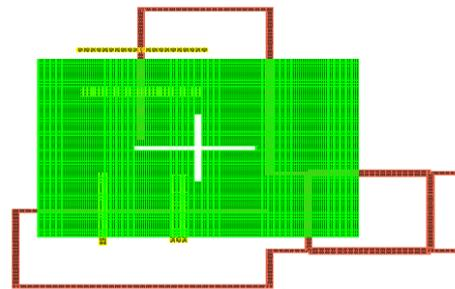
Figure-5: Structure of Complete design of antenna using hybrid coupler with CSRR
