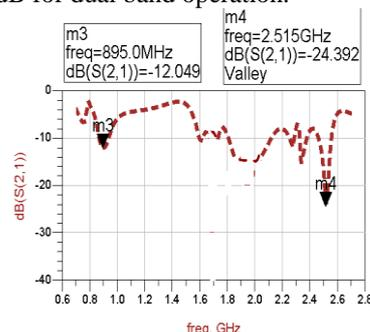
Figure-7: Isolation loss measurement
