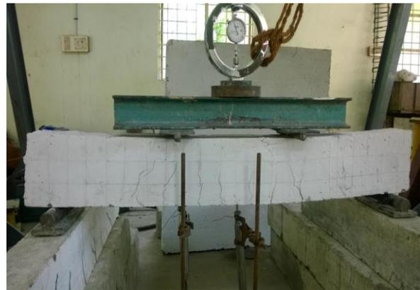
Fig-10 Failure pattern of the conventional beam
