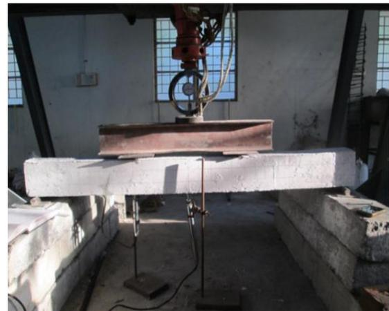
Fig -6: Testing of RC Beam (80% Sea sand)
