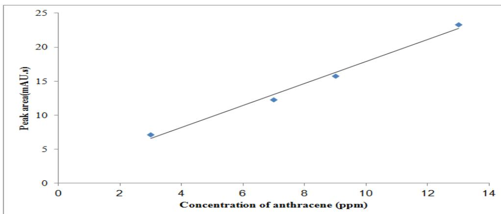
Figure 3: Calibration curve of standard anthracene compound.
