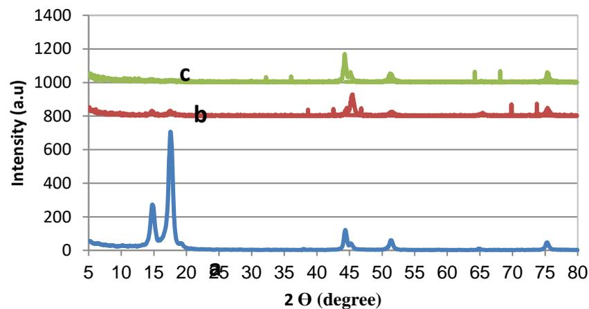
**Figure 1:** XRD plots of (a) HA, (b) HA-Ti and (c) HA-Ti-Ag coatings
