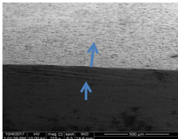
**Figure 3:** SEM micrograph of the HA-Ti-Ag coating-metal interface. Blue arrows showing coating thickness.
