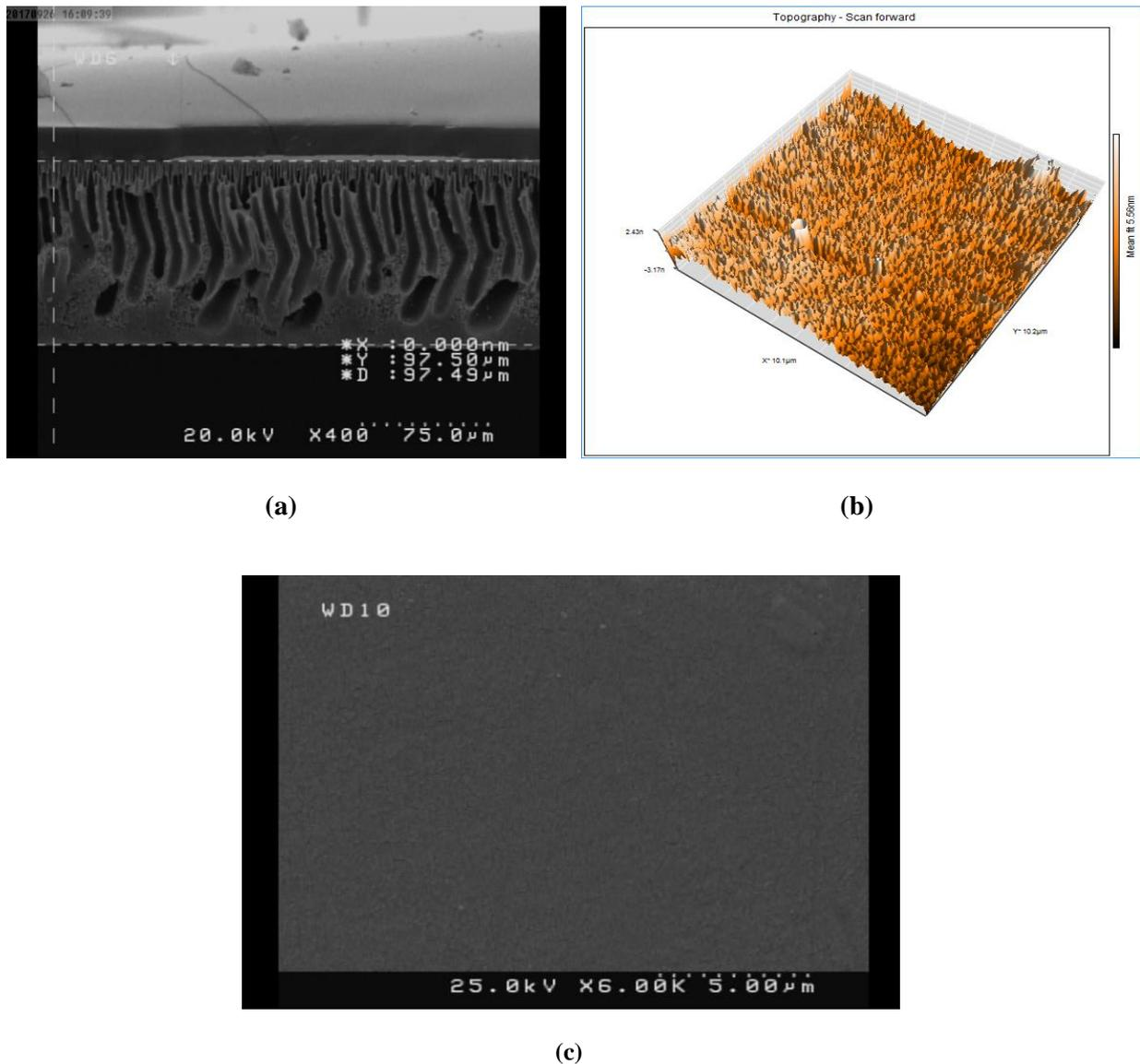
**Fig. 2: Characteristics of PDMS/PES composite membrane: (a) Cross sectional FESEM image, (b) Surface AFM image and (c) top FESEM image**
