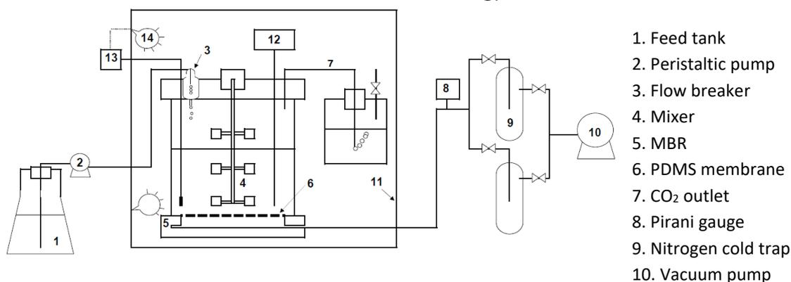
**Fig. 1. Schematic diagrams of MBR pervaporation system for fermentation (Najafpour, 2015)**
