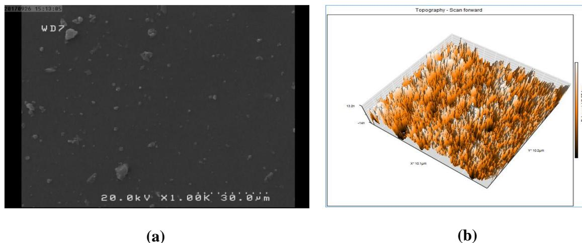
**Fig. 3: Characteristics of surface coated by SiO<sub>2</sub> on PDMS/PES composite membrane: (a) top surface FESEM image, (b) Surface AFM image**
