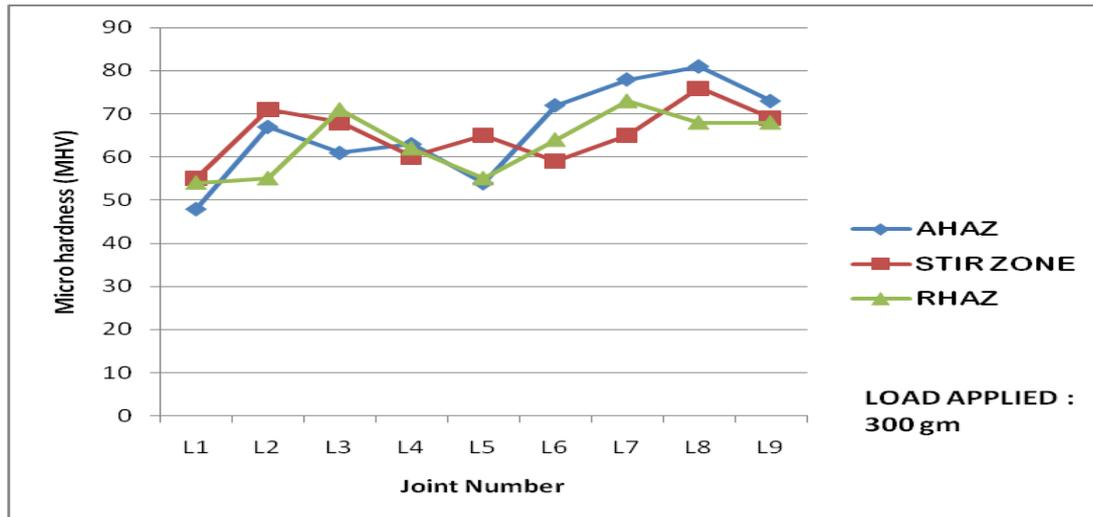
FIG II: Comparison of Micro hardness values taken at AHAZ, Stir Zone, RHAZ
