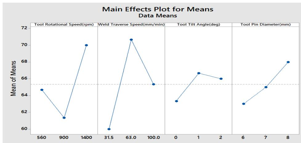
Fig VI: Process Parameters (Input Responses) Vs Mean of Means (Output Response) Plot.
