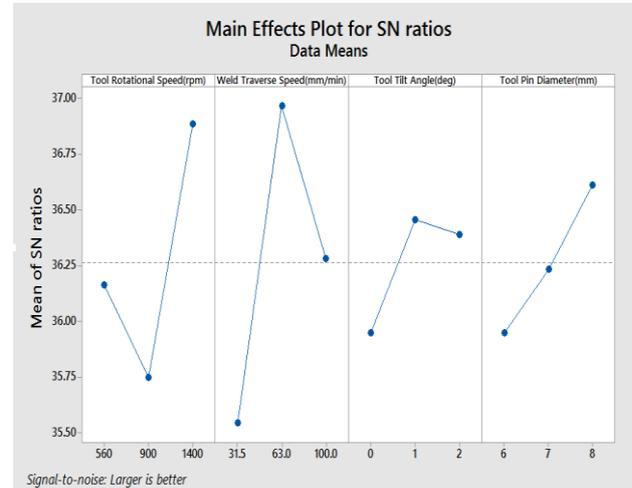
Fig V: Process Parameters (Input Responses) Vs SN Ratio (Output Response) Plot.
