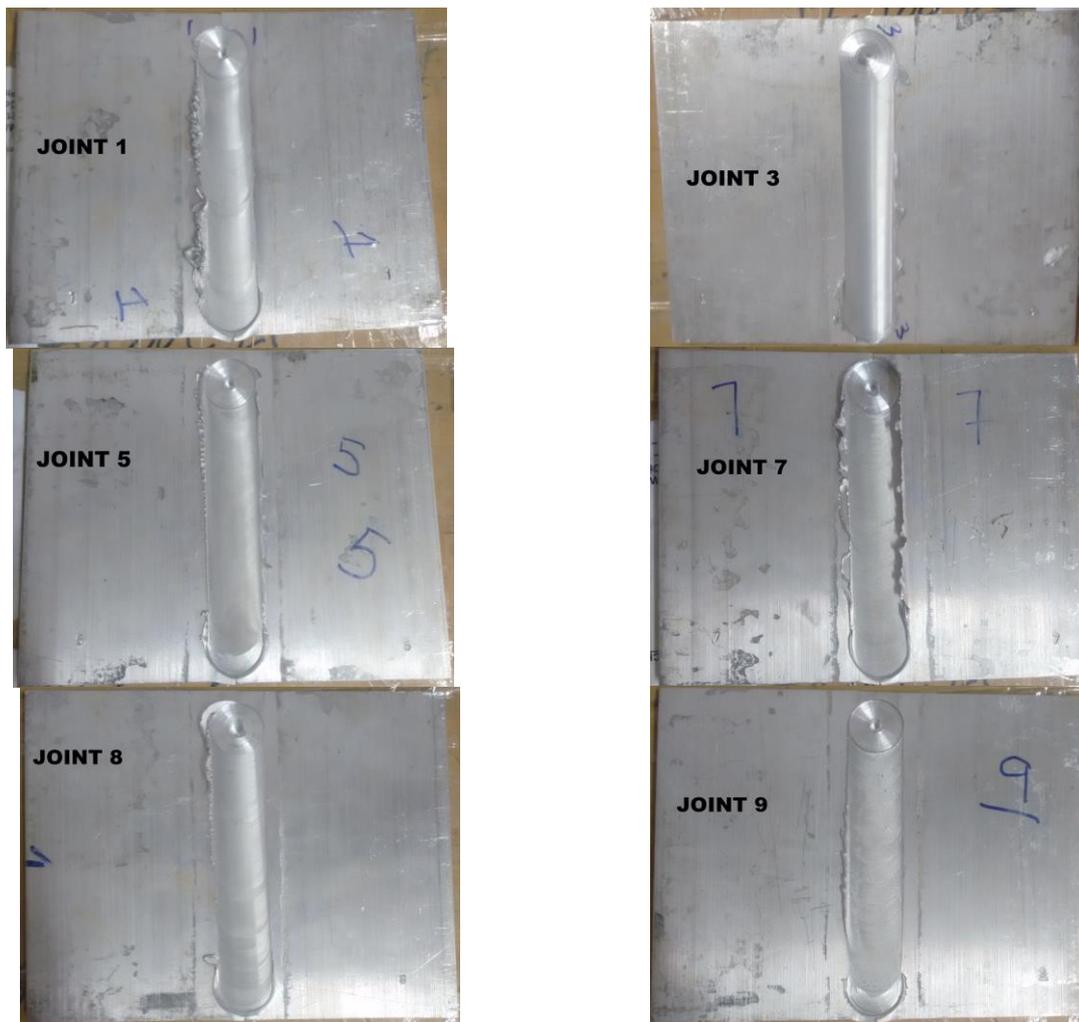
Fig I: Post welded joints 1, 3, 5, 7, 8, 9
