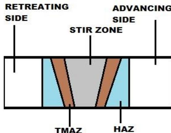
Fig IV: Different weld zones in FSW.
