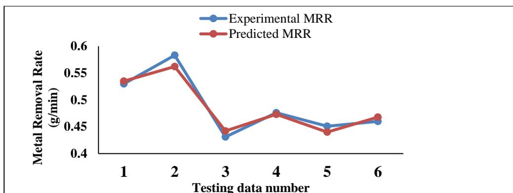
Fig. 7: Comparison for the testing data of metal removal rate
