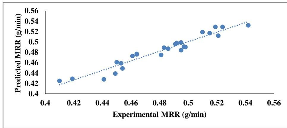
Fig. 8: Scatter plot for the training data of metal removal rate
