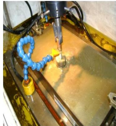
Fig. 2: Jet flushing system in spark erosion machining
