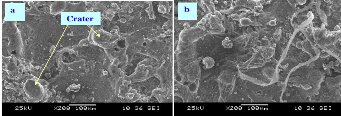
Fig. 4ab: SEM photograph of spark erosion machined surface of Al 6061 composites reinforced with SiC and graphite particles at a voltage 50V and a flushing pressure 3psi: a) 3A,400µs, b) 15A,400µs
