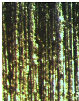
Fig. 1: The surface of the steel samples after mechanical processing (× 100).
