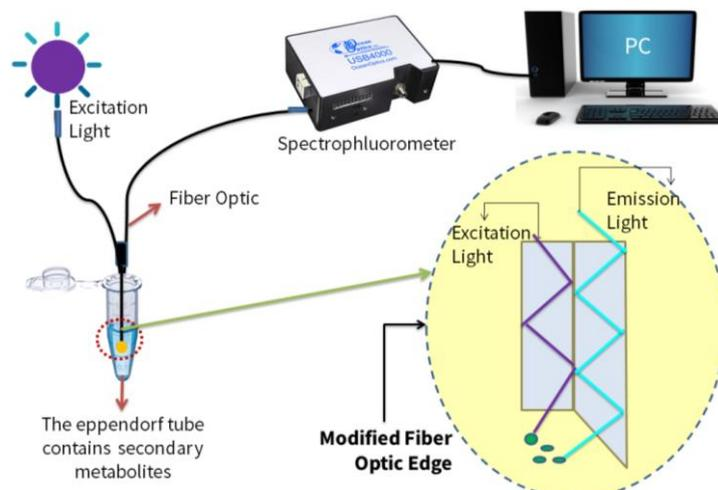
**Fig. 1:** Pathogenic fungi detection scheme on rice seed by fiber optic fluorescence spectroscopy
