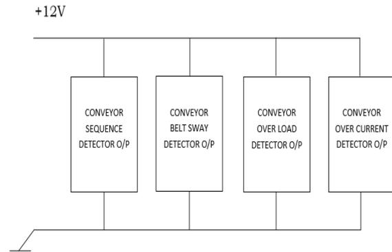
Figure-3: Split up of conveyor system
